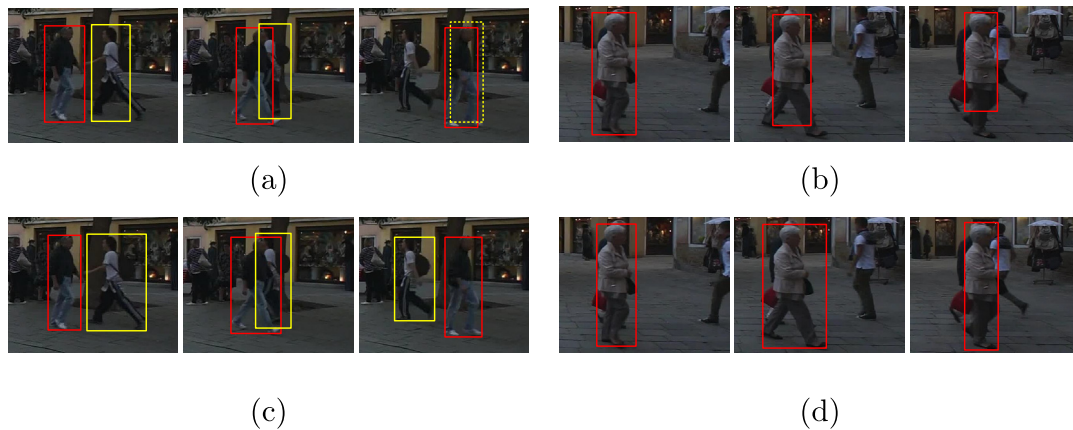
Fig. 1. Inaccuracy tracking results and modified results. The tracking drift (a) and the scale bias (b) occur when adopting CF tracking directly in the MOT task. These problems are fixed by our method (c) and (d).
